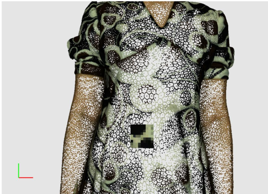
Color patch construction on 3D point cloud of a scanned woman
